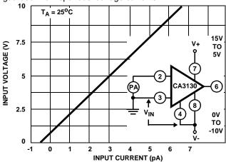
FIGURE 3. INPUT CURRENT vs COMMON-MODE VOLTAGE
