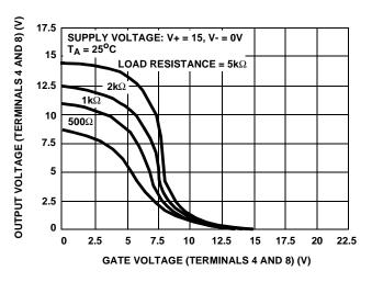
FIGURE 2. VOLTAGE TRANSFER CHARACTERISTICS OF CMOS OUTPUT STAGE
