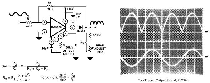
Top Trace: Output Signal; 2V/Div. Bottom Trace: Input Signal; 10V/Div.  $R_3 = 4k\Omega \left(\frac{0.75}{0.5}\right) = 6k\Omega$ Time base on both traces: 0.2ms/Div.
