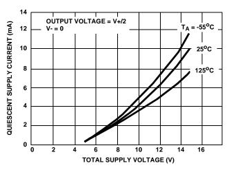
FIGURE 21. QUIESCENT SUPPLY CURRENT vs SUPPLY VOLTAGE
