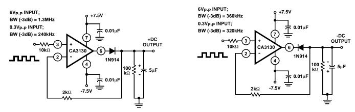
FIGURE 12A. PEAK POSITIVE DETECTOR CIRCUIT
