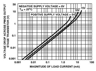
FIGURE 22. VOLTAGE ACROSS PMOS OUTPUT TRANSISTOR (Q<sub>8</sub>) vs LOAD CURRENT
