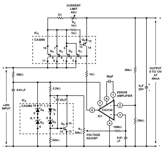
REGULATION (NO LOAD TO FULL LOAD): <0.01% INPUT REGULATION: 0.02%/V HUM AND NOISE OUTPUT: <25 $\mu$ V UP TO 100kHz
