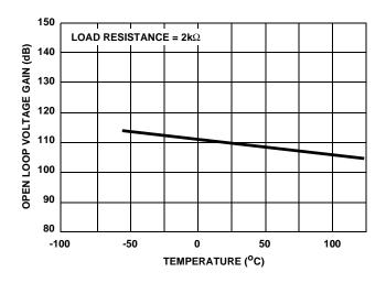
FIGURE 18. OPEN LOOP GAIN vs TEMPERATURE
