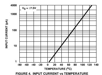
In applications requiring the lowest practical input current and incremental increases in current because of "warm-up" effects, it is suggested that an appropriate heat sink be used with the CA3130. In addition, when "sinking" or "sourcing" significant output current the chip temperature increases, causing an increase in the input current. In such cases, heatsinking can also very markedly reduce and stabilize input current variations.
