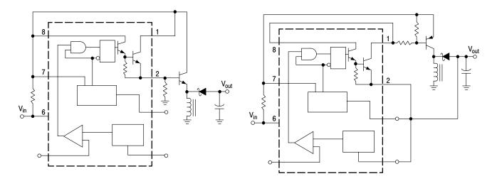
Figure 12. External Current Boost Connections for I<sub>C</sub> Peak Greater than 1.5 A12a. External NPN Switch12b. External PNP Saturated Switch
