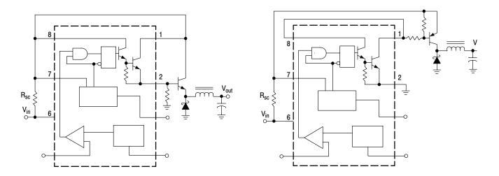
Figure 10. External Current Boost Connections for I<sub>C</sub> Peak Greater than 1.5 A
