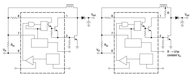
Figure 8. External Current Boost Connections for I<sub>C</sub> Peak Greater than 1.5 A
